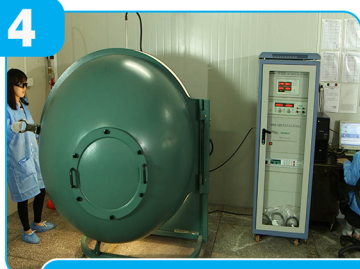
LED Light Source Inspection
