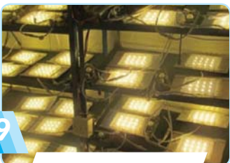
Automatic Aging Process for 24 hours
