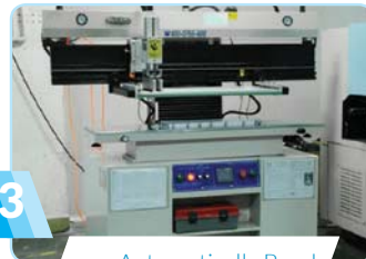
Automatically Brush Soldering Paste on PCB
